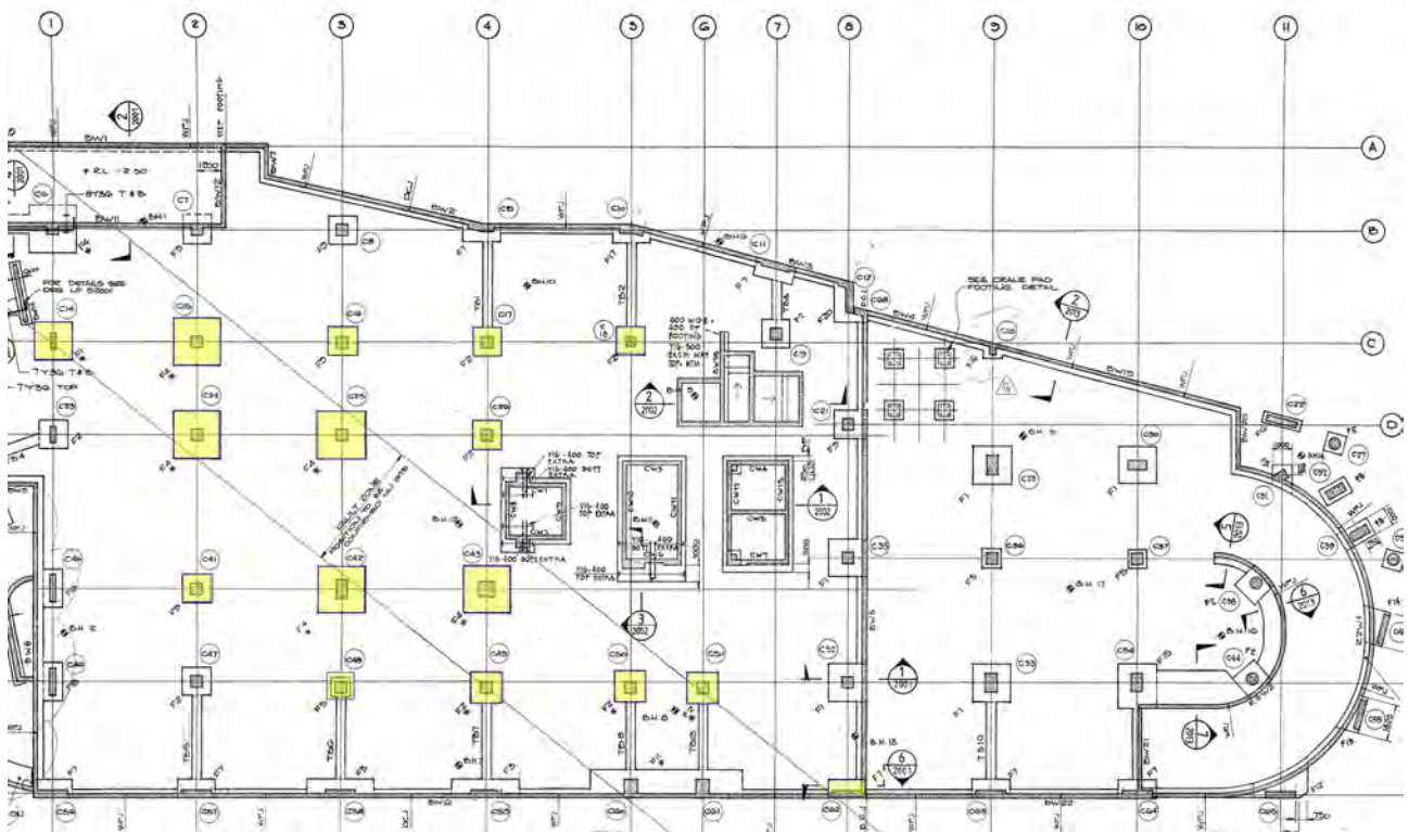
As noted in the Douglas Partners report, there remains a risk of variability in strength under each specific footing, and it is recommended that investigations of founding material beneath all footings is carried out prior to construction works progressing to manage this risk.
